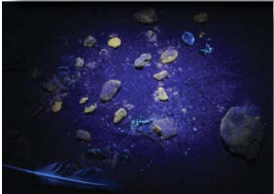
Tar balls and beach debris under the LVUV light. Note the bright orange of the tar balls.
